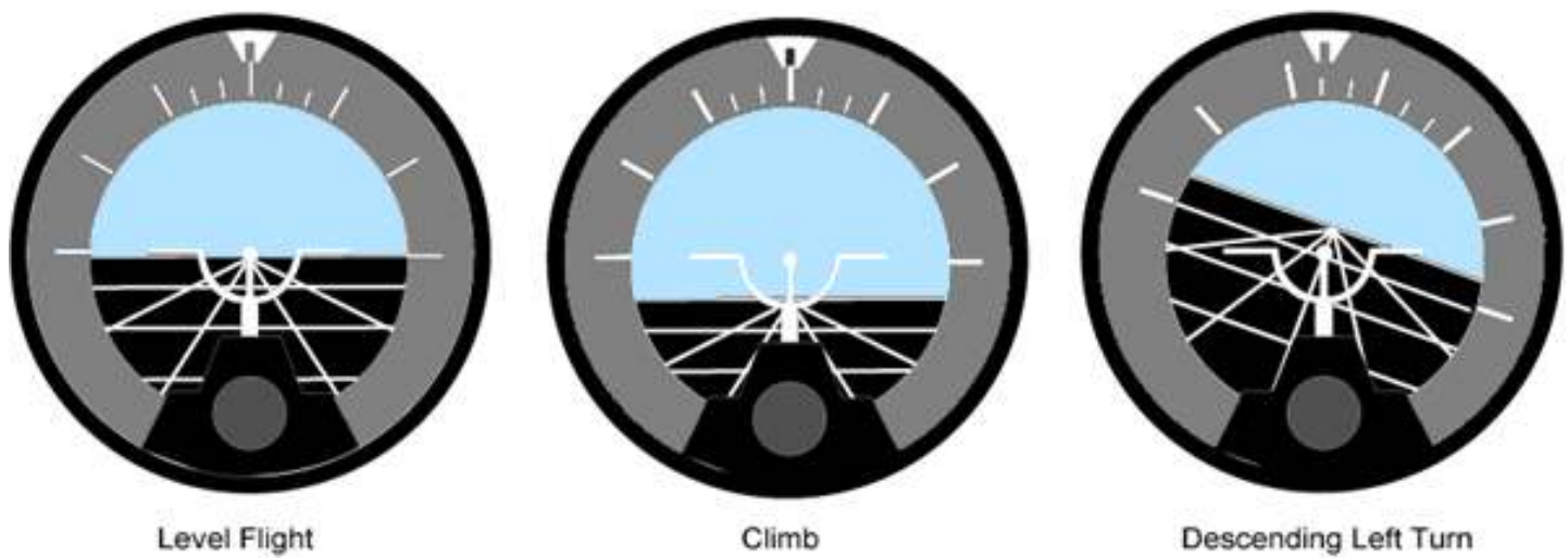
Figure 3-11.—Various indications on the attitude indicator.
