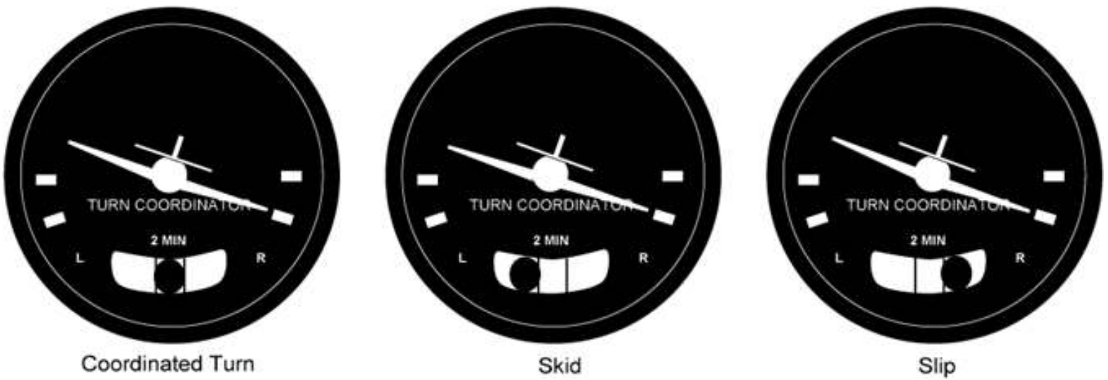
Figure 3-8.—Turn coordinator indications.
