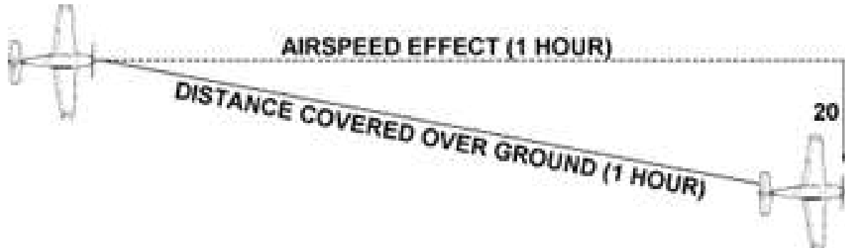
Figure 8-13.—Airplane flightpath resulting from its airspeed and direction, and the windspeed and direction.
