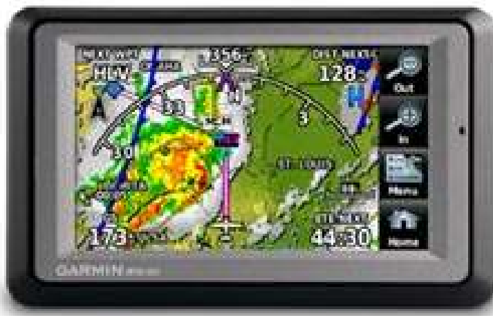
Fig 8.31 Garmin™ Handheld GPS unit with moving map display and nav data
