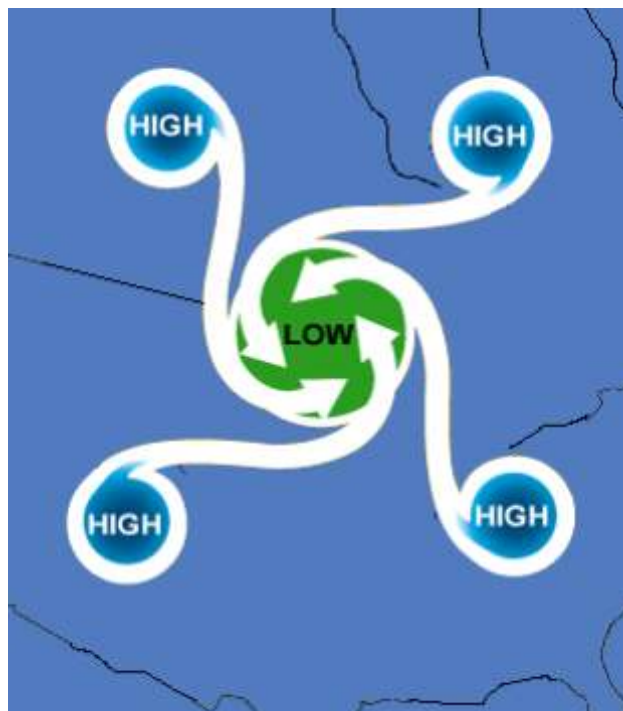
Figure 5-7.—Circulation of wind within a “low.”
