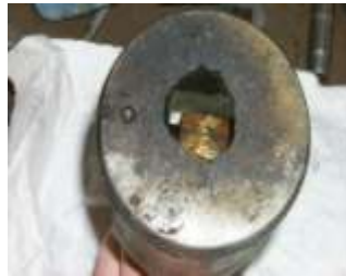
Piston damaged by detonation
