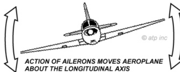
Figure 1-30.—Effect of ailerons.
