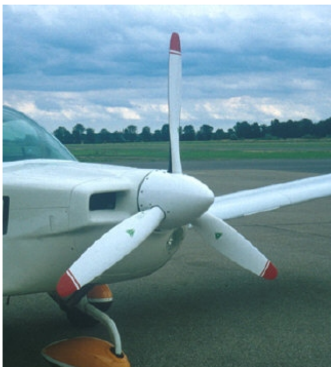
Each blade of a propeller presents a different Angle of Attack to the oncoming airflow
